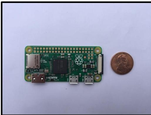
The objective of the project was to have a product available for under US \$30. This Raspberry Pi circuit board would include all of the options to be used as a fully operational computer, including general purpose processing capabilities, RAM -
